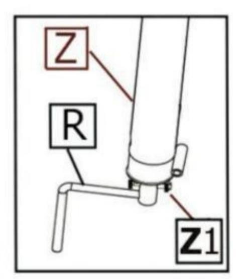
Handle (R) can be removed or stored by removing small
