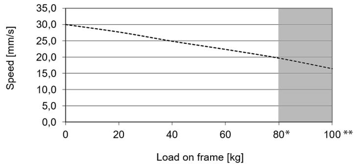
Above curve applies to a centrally placed load and is only valid in respect of duty cycle: 10% by 50% of max. working load or max. 2 min. continuously.
