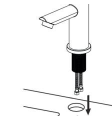
3. Place the tap with the installation tube in the tap hole.
