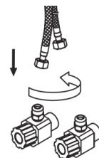
6. Wrap plumber's tape around the tap threads. Connect the flexible connections (8&9) to the angle valves and tighten them.
