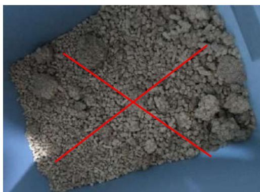
Agglomeration of poor-quality pellets
