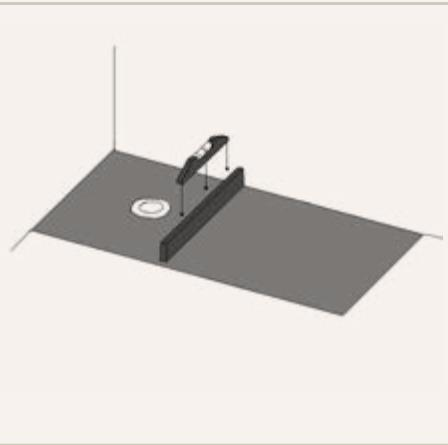
Spread evenly and check the level at the same time. Wait for the mortar to set well according to manufacturer's specifications. Check the level is correct once the product is completely dry.
