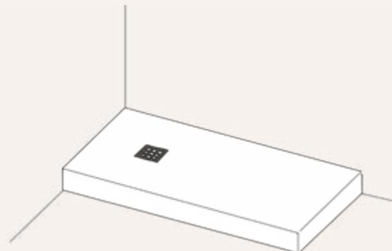
Check before installing the new shower tray that it is in good condition and that the installation surface has no defects.
