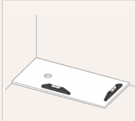
Place the shower try and let the product set according to the manufacturer's specifications. Put the wall cladding. Finish the valve installation. Check level. Check with water that the shower tray drains properly.
