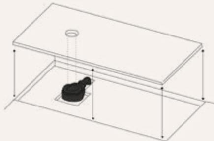
Check that the shower tray is well positioned and the valve corresponds with the shower tray hole.
