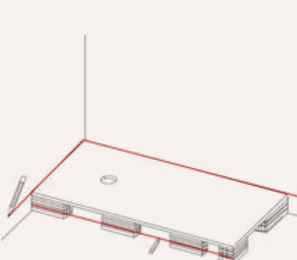
Raise the tray using bricks to the desired height. Draw the line where the tray and the position of the bricks will remain. For a proper setting and sealing, no tiling are required for the first row of tiles.
