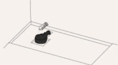
Install the valve according to the manufacturer's specifications and connect it to the PVC drain pipe. Check for leaks.
