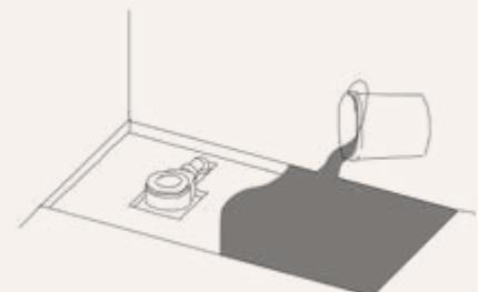
Check that the base is level, clean and free from debris. Place the mortar in case you need to level the area.
