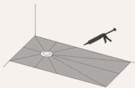
Spread it quickly and uniformly before the sealant acts and dries.
