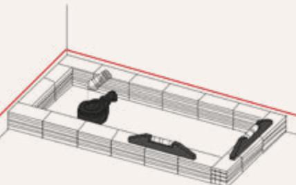
Check that the shower tray is well positioned and the valve corresponds with the shower tray hole.
