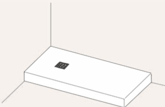
Check before installation that there are no defects on the surface of the shower tray and that it is supported on a flat surface and positioned horizontally.
