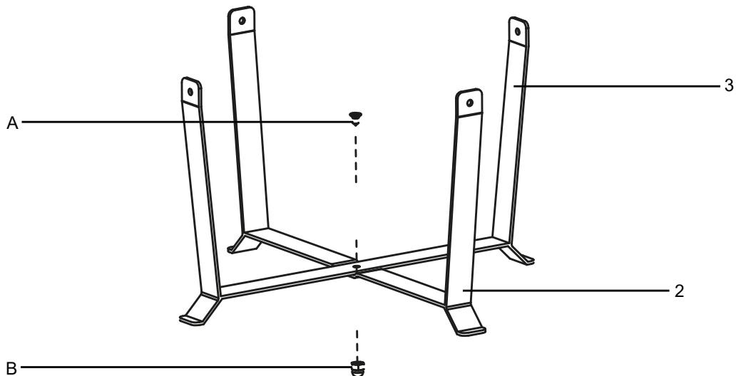
**STEP 2:** Attach the bracket from Step 1 to the brace ring (1) using 4 screws (A) and 4 dome-headed nuts (B).
