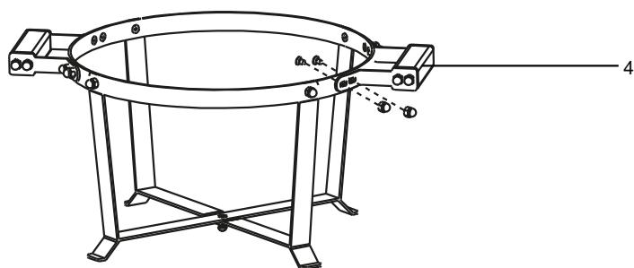
**STEP 3:** To attach the two handles (4) to the lid of the brace ring (1), align the bolt holes on the handle with the pre-installed bolts on the lid. Secure the handle (4) using the 4 pre-attached dome-headed nuts (B).
