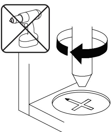
**EN** Turn cam lock clockwise to tighten.
