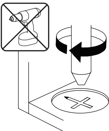
**EN**\_Turn cam lock clockwise to tighten.
