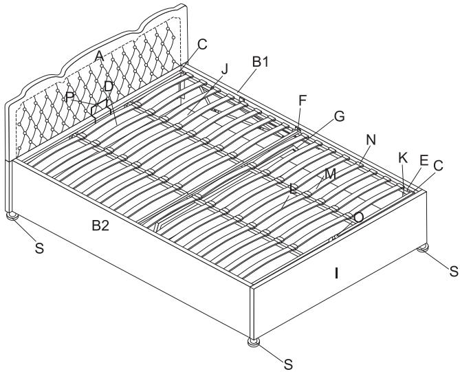
Notice: Do not tighten the screws too tightly at the beginning of the assembly. After each hole position is matched well, with gently force to screw, if there is no problem, then tighten all the screws.
