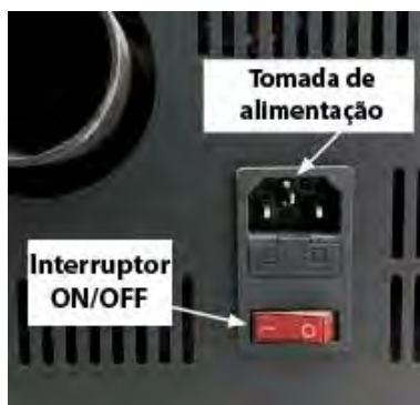
Tomada elétrica/interruptor ON/OFF
