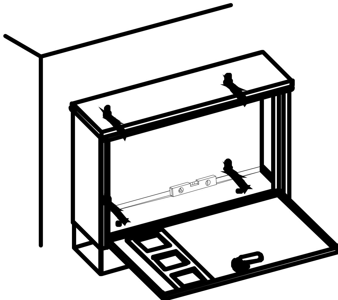
**EN** If it is a solid wall, please use expansion and self-tapping screws, if it is a wooden wall, only use self-tapping screws, please do not overtighten the screws
