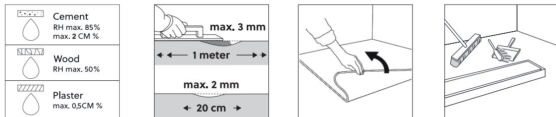
The subfloor must be completely dry when installing on :
