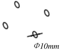
Step3: Insert the metal expansion tubes(C) into the drilled holes.
