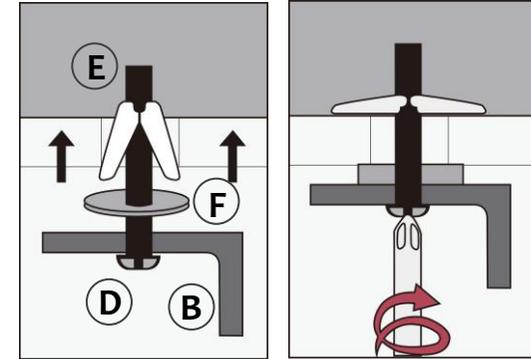
Step4: Tighten the screws .
