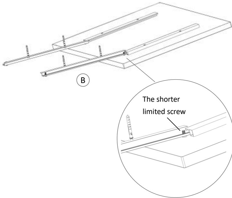
2. Make the completely fall between the two limited screws, and the installation is completed.
