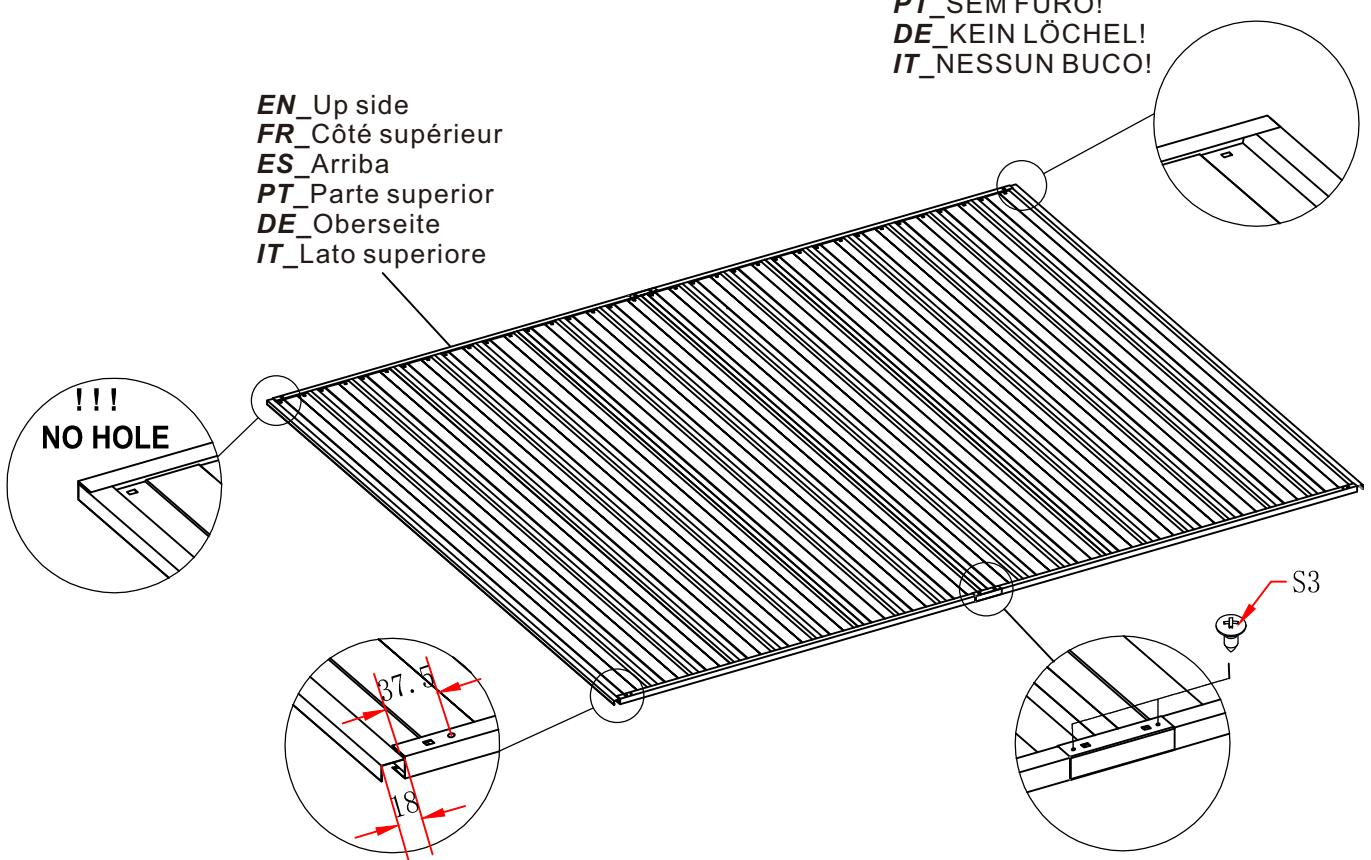
**EN**\_Noted: Drill S3 on both sides to improve the stability of connector
