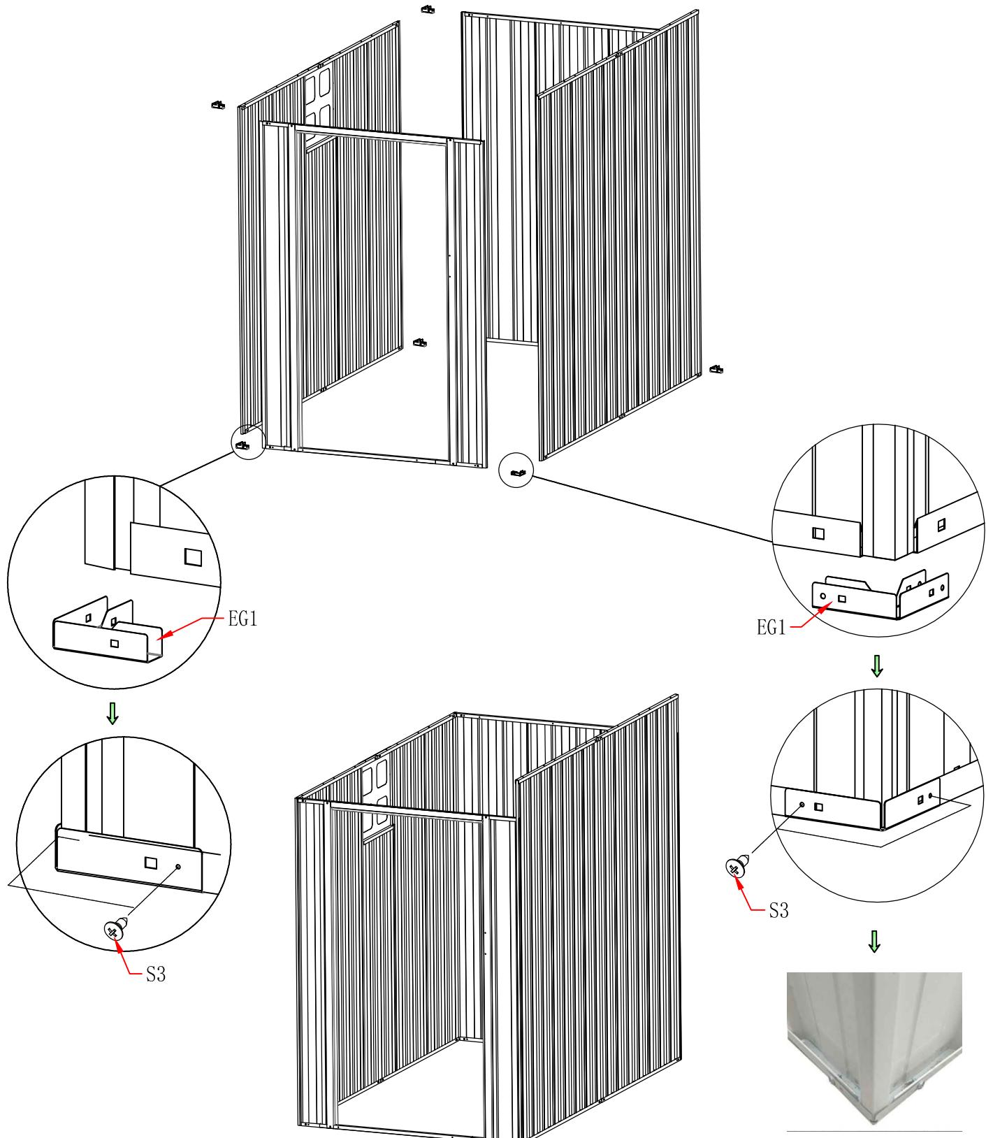
**ANCHORING ASSEMBLY/ASSEMBLAGE D'ANCRAGE/
