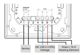
**Important:** An external temperature sensor must be connected for proper device operation. The indicator LED will flash green if no sensor is detected.
