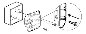
4. Confirm the position of the device buckle.
