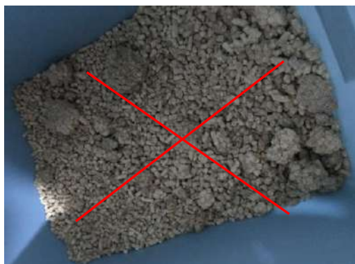
Agglomeration of poor-quality pellets
