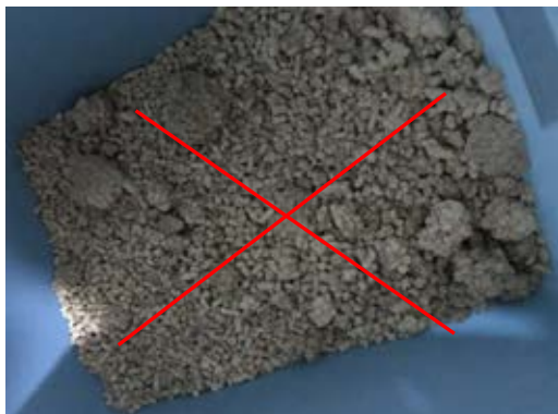
Agglomeration of poor-quality pellets
