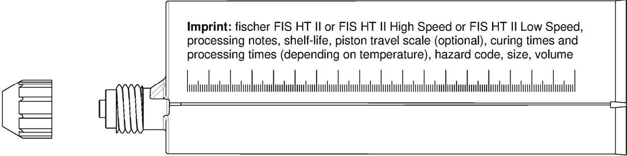
**Injection cartridge (coaxial cartridge) with sealing cap; Sizes: 100 ml, 150 ml, 300 ml, 380 ml, 400 ml, 410 ml**
